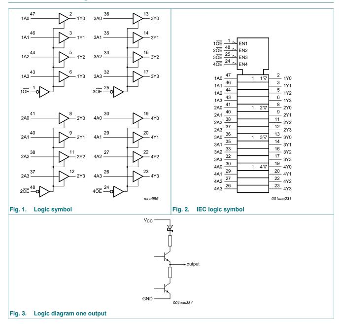
16-bit buffer/line driver with 30  $\Omega$  series termination resistors; 3-state
